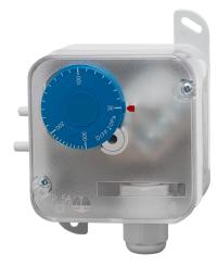
PS differential pressure switches are designed for monitoring over and under pressures and pressure differences in systems that handle air and other non-aggressive gases. PS switches offer a cost-effective solution for filter, fan and duct pressure monitoring for building automation systems. The switching point can be adjusted manually.
