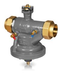
The PCMTV DN32-50 valves are temperature control valves with full authority over the entire flow range and measuring ports. This means that each individual terminal receives the flow required even in part load conditions. The PCMTV valves do not require any setting ratio calculation or valve authority calculation.
