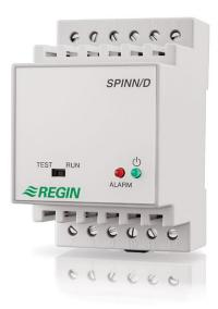
SPINN/D is an electronic rotation sentinel intended for supervision of rotary heat exchangers in air handling systems. The rotation sentinel will give an alarm at an unplanned stop of the heat exchanger wheel. SPINN/D Rotation sentinel for heat exchangers
