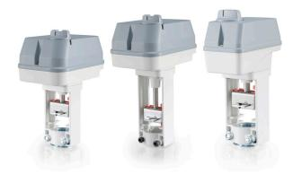
Valve actuator for control of Regin's range of valves. Available in models with actuator force of 500, 1000, 1800 or 2500 N. The actuators can be operated manually with the manual override mechanism on the lid. Using an adapter kit, the actuator can also be adapted for use with other valves on the market.
