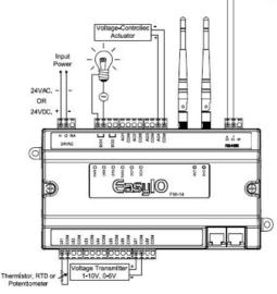
The FW-14 comes with one standard RS485 driver to support BACnet MSTP Client. The FW-14 also comes with two Ethernet Ports to program the Sedona Application, TCOM, FGP2P, BACnet and for web configurations.
