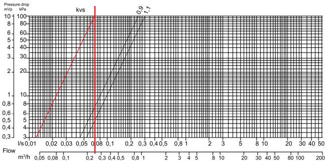
The valves have adjustable kvs value (kvs = the flow in m3/h at a pressure drop of 100 kPa).
