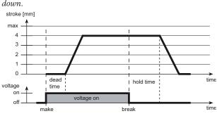
\* This applies to valves that close when the stem is pushed down.
