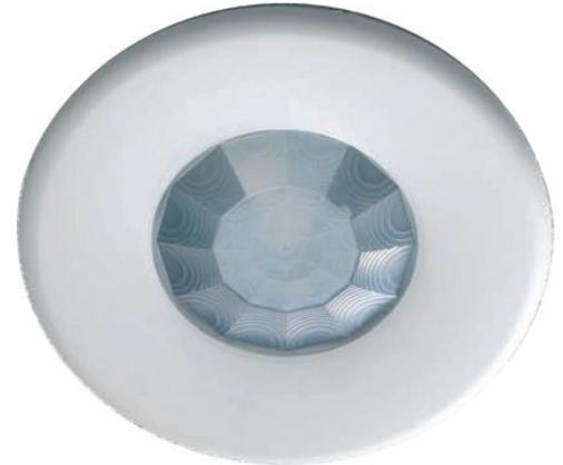
Retractive spring clips enable the sensor to be mounted easily from below within thin perforated-metal ceilings and thicker plaster ceilings while the body incorporates integral cable-retention clips.
